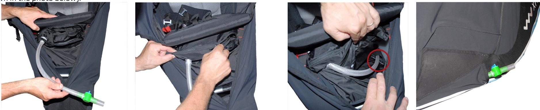
The ballast compartment under the instrument holder operates in approximately the same manner. Open the zip of the fabric flap, which becomes the ballast bag container. Place the ballast bag into position so that the drain tube is in correspondence with the eye. Run the drain tube between the seat angle adjustment strap and the main harness strap, and then pass it out of the harness.
