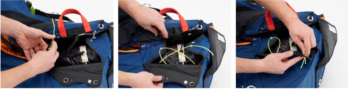
Introduce the handle's metallic pins into the elastic loops and under the transparent cover. The cord must absolutely be removed at the end of this phase, and must be extracted slowly in order to avoid damaging the elastic loops due to excessive friction between the parts. In the end the zip should be completely closed until introducing the zip pull under the cover behind the left shoulder-strap.
