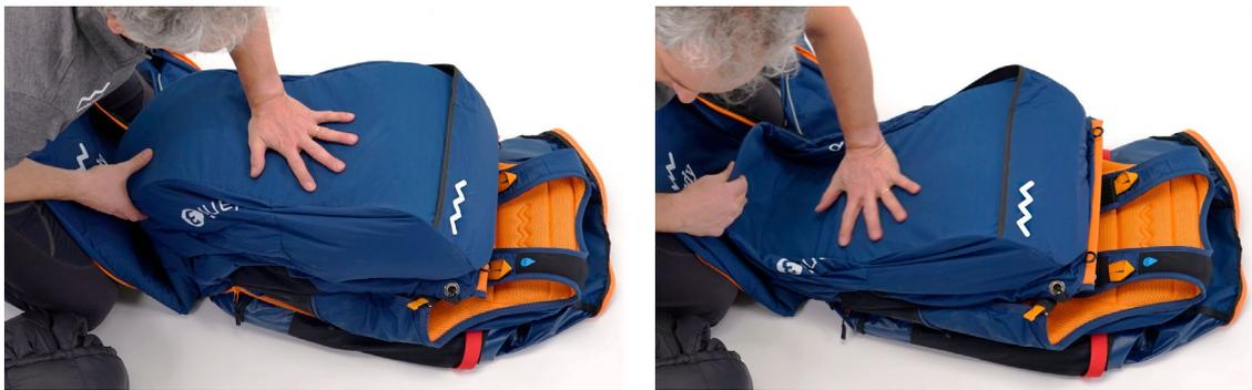
Put the previously folded paraglider above the harness airbag. Place the paraglider above the rear pocket and, finally, close the backpack.
