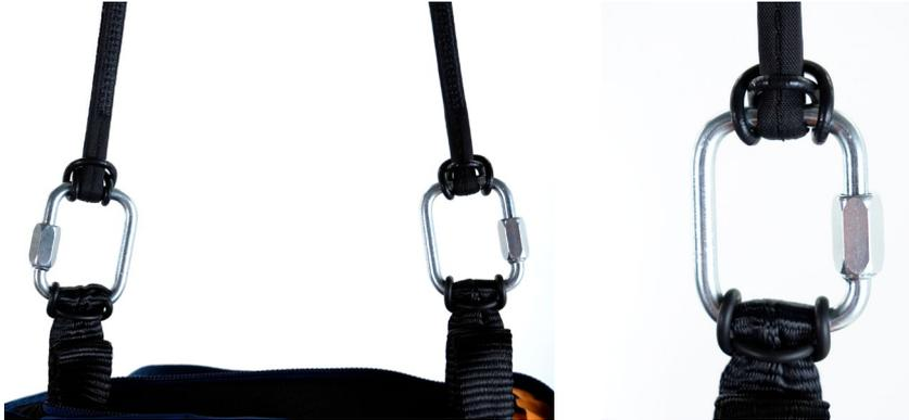
The two connections should be made using screw-lock karabiners with a breaking strength of at least 1,400 kg. In any case, it is important to verify that the length of the bridle is sufficient to position the reserve parachute inside the harness pocket, and that there is sufficient play to enable the parachute to be taken out of the pocket without causing the reserve parachute deployment bag itself to open during extraction.
