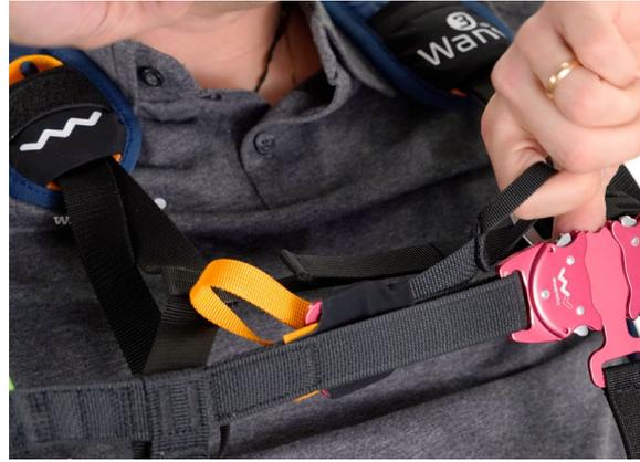
asymmetric collapse of the sail. There is also a second strap which lets you adjust the distance between the shoulders which, in case you forget to fasten the chest, prevents the pilot from falling out.
