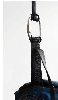
The two connections should be made using screw-lock snap-hooks with a breaking strength of at least 1,400 kg. It is important to make sure that the bridle is long enough to position the reserve parachute inside the harness pocket and that there is sufficient room to take the parachute out of the pocket without causing the reserve parachute deployment bag itself to open during extraction.
